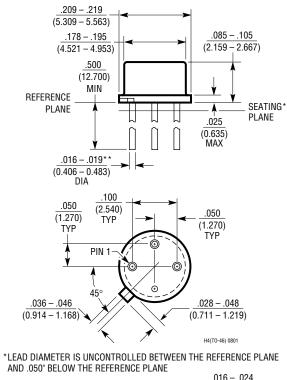
\*\*FOR SOLDER DIP LEAD FINISH, LEAD DIAMETER IS  $\frac{.016 - .024}{(0.406 - 0.610)}$
